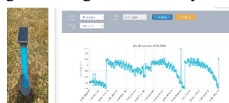
Figure 1. Low cost IoT sensor based (left) water level monitoring device, and (right) water level data to monitor AWD irrigation practices
