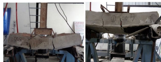
Figure 4. Failure pattern of gird strengthened specimens
