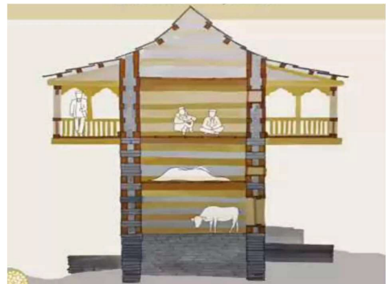
Figure1. Typical section of Kath Kuni style house
