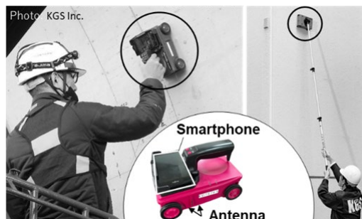
Figure 1. Smartphone-equipped handheld GPR used in this study
