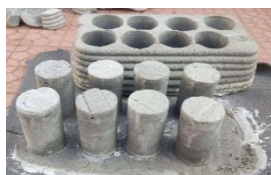
Figure 7. Printed concrete bed and extracted core samples
